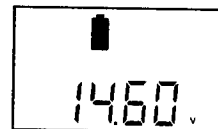
Fig 20. battery over voltage setting
