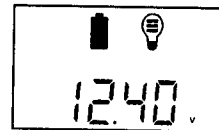
Fig 19. battery low voltage return value setting
