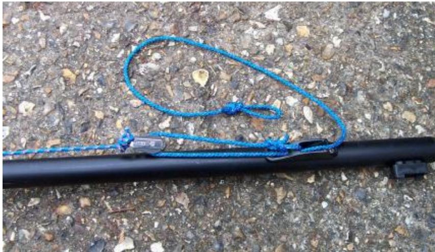
Picture 4.23 The rudder downhaul fitted.
