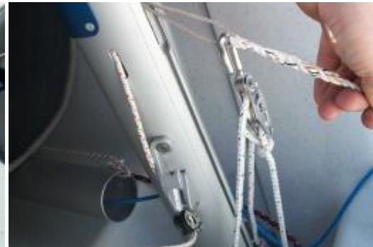
Picture 4.20 Connecting the rig tension.
