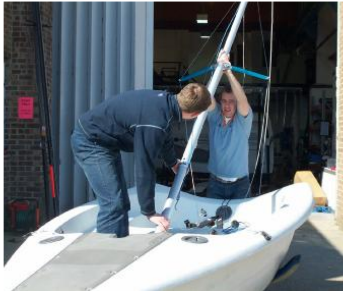
Picture 4.7 Raising the mast.
