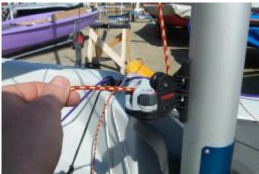
Picture 4.15 The gnav control line.
