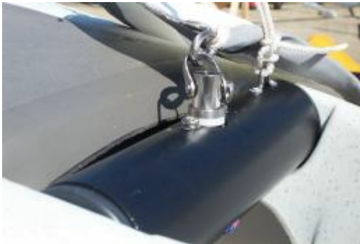
Picture 4.17 The tack of the jib
