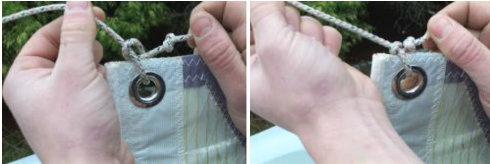
Picture 4.27 Tying the main halyard.
