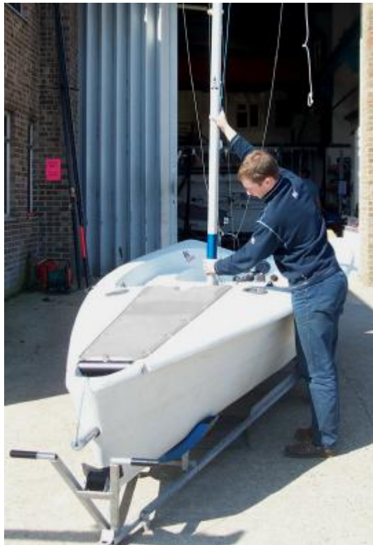
Picture 4.5 Stepping the mast single-handed.
