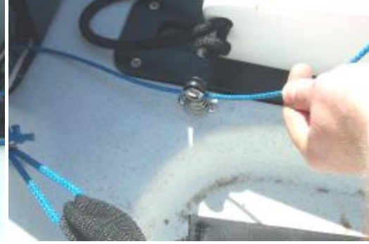
Picture 4.12 The spinnaker downhaul block.
