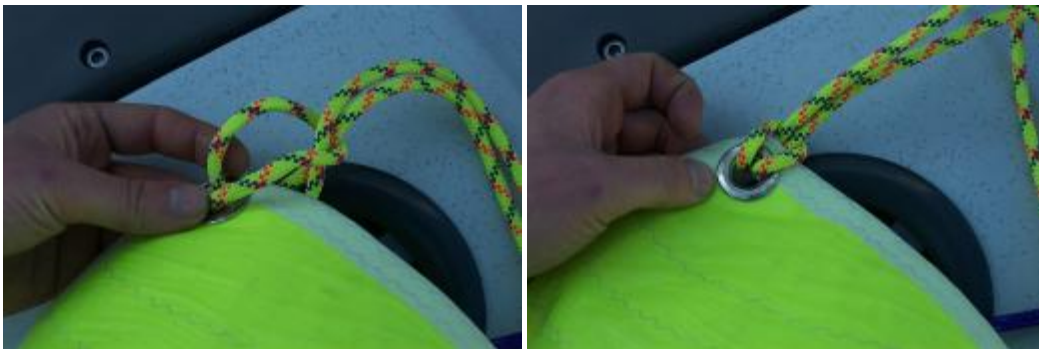
Picture 4.35 Tying the spinnaker sheets.
