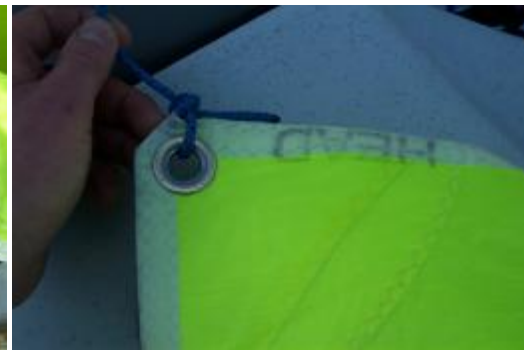
Picture 4.32 The head of the spinnaker.
