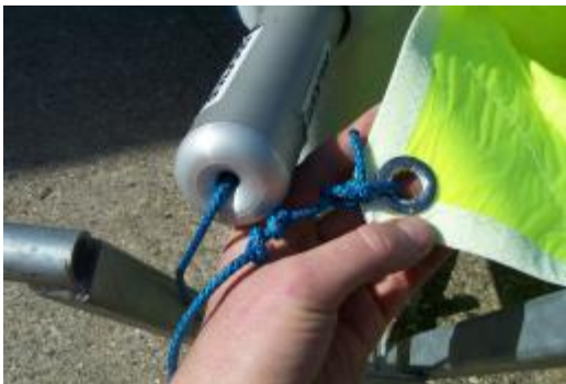
Picture 4.31 The tack of the spinnaker.
