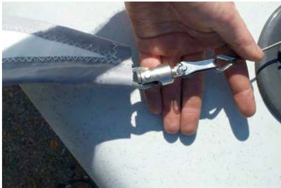
Picture 3.19 The Head of the Jib Attached
