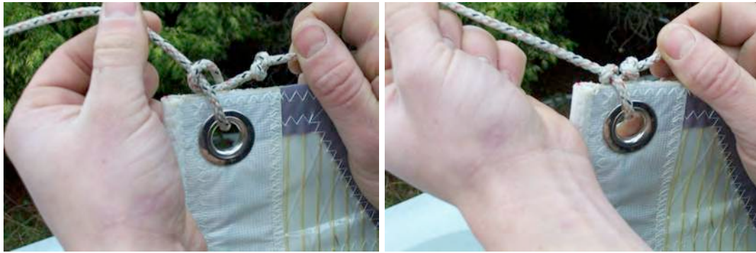
Picture 3.27 Tying the Main Halyard
