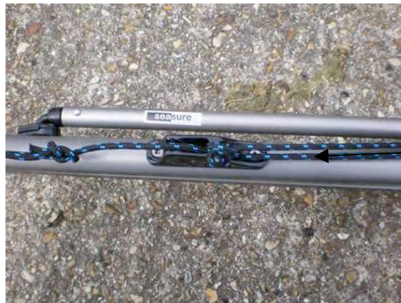
Picture 3.23 The Rudder Downhaul
