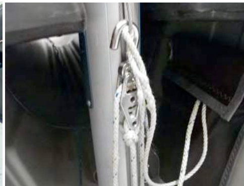
Picture 3.20 Connecting the Rig Tension
