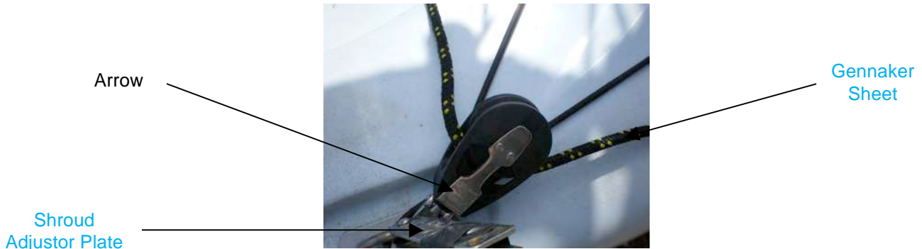
Picture 3.36 The Gennaker Sheet Block
