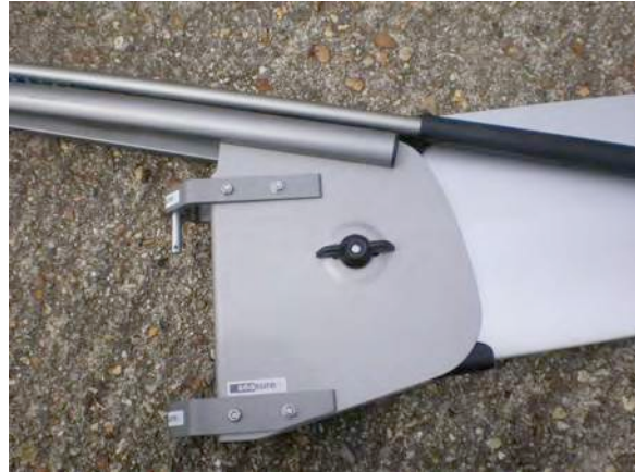
Picture 3.22 The Rudder Fitted in the Stock
