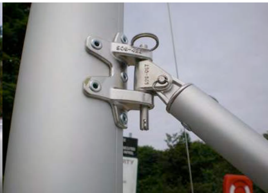
Picture 3.14 Connecting the Gnav to the Mast
