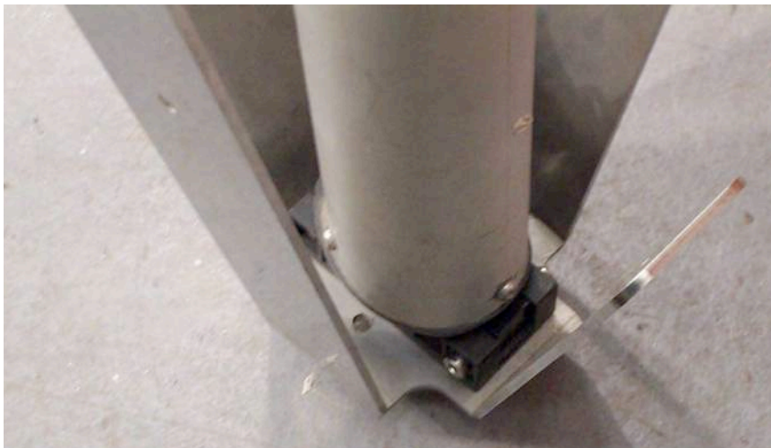
Picture 3.4 The Mast Foot Correctly Located
