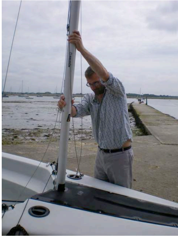
Picture 3.5 Stepping the Mast Single Handed
