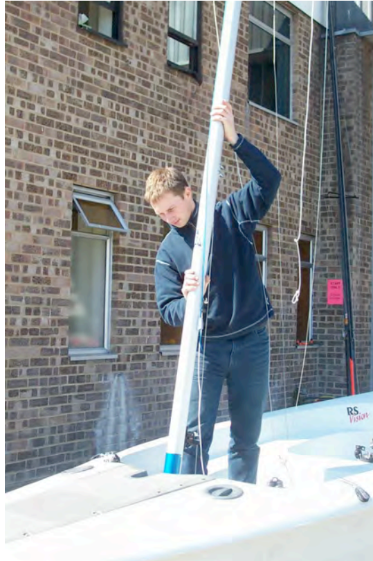
Picture 3.8 Stepping the Mast
