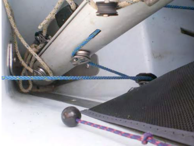
Picture 3.10 Threading the Gennaker Halyard
