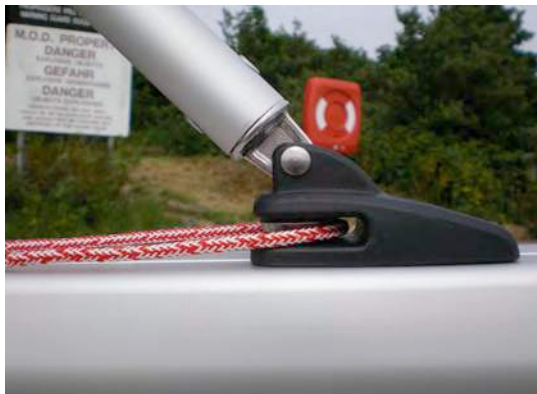
Picture 3.13 Connecting the Gnav to the Boom
