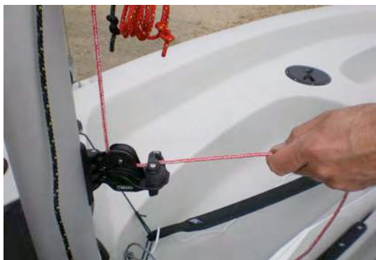
Picture 3.15 The Gnav Control Line
