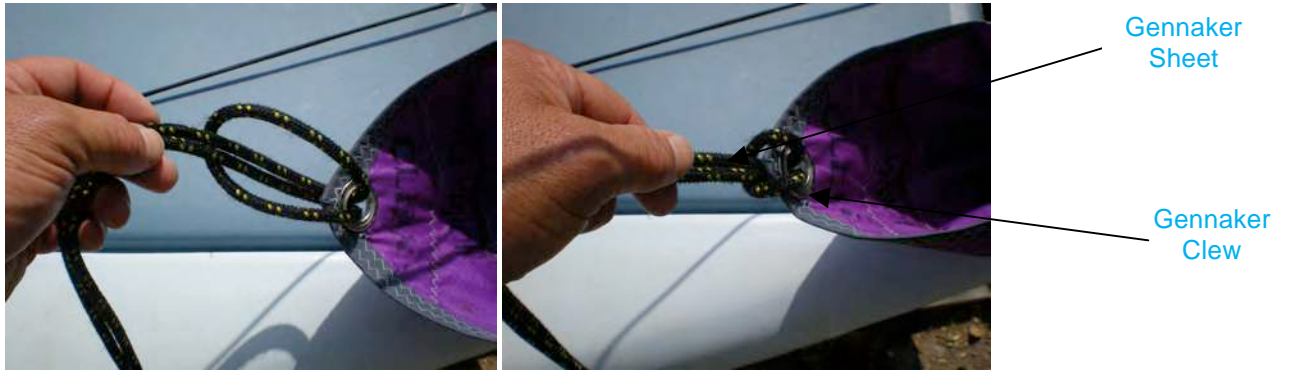
Picture 3.35 Attaching the Gennaker Sheet
